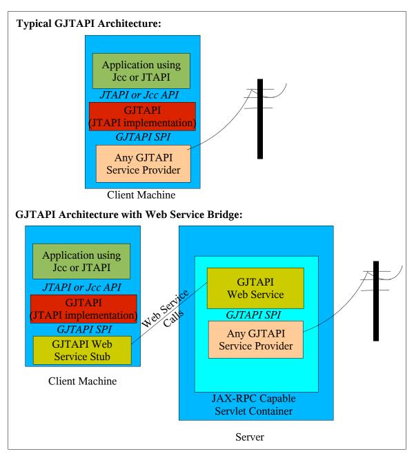
Basically, the Web Service Bridge is an adapter that delegates GJTAPI service-provider-interface calls on to a remote GJTAPI service provider. By adherring to the GJTAPI SPI on both ends, the Web Service Bridge can be injected anywhere in the GJTAPI application stack to allow access to a service provider on a remote machine.
